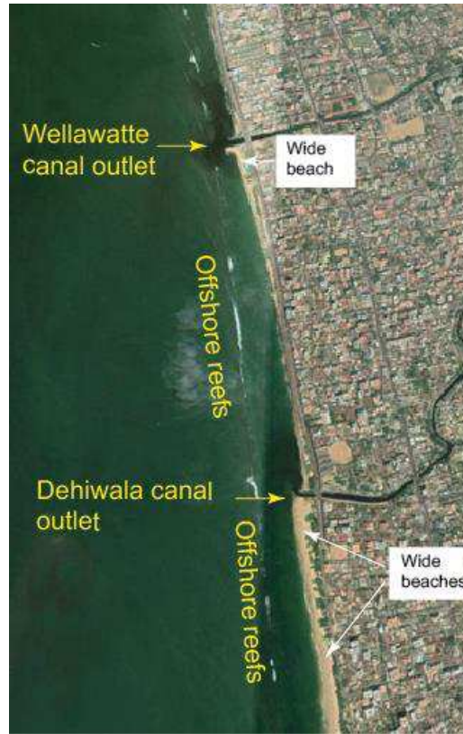
Figure 5 –Dehiwala and Wellawatte Canal outlets
